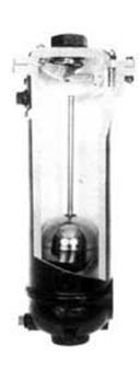
he Universal Sewer Air Release Valve is designed to permit the automatic escape of large quantities of air from a pipeline when the line is being filled, and to permit air to enter the pipeline when the line is being emptied.
