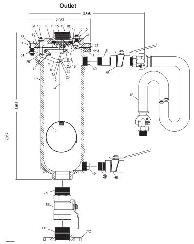
Note: Inlet Gate Valve is included when backflushing attachments are provided.
