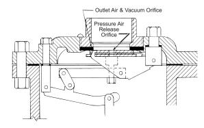
All CRISPIN Air and Vacuum Valves have standard Buna-N seating material with a Shore durometer of 70-80.
